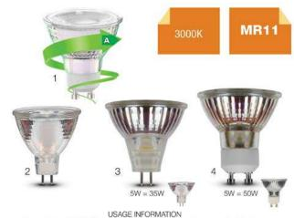
Compatible with 12V AC output electromagnetic transformers and with drivers for LEDs and with constant current drivers. Do not use with dimmers. Do not use these items with electronic transformers for halogen lamps.
