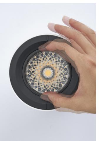
**ZOOM Smart** A manual zoom optic composed of two elements operating together which makes it possible to vary the beam opening by rotation. The optical system is housed entirely inside the projector body and guarantees excellent performance and precise beams.
