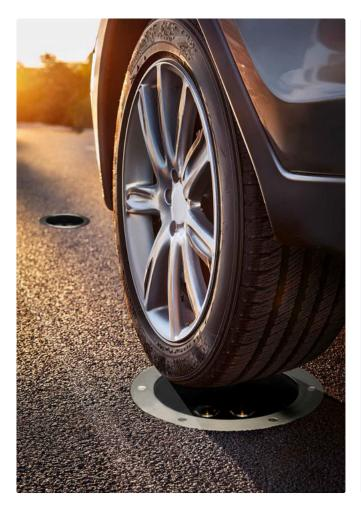
Drive-over range The entire Keplero range is walk-over and drive-over (IK10) in compliance with EN 60598-2-3 regulation. Resistant to high pressure washing The glass has a "C" shaped gasket that surrounds it and perfectly isolates the optical chamber to ensure an IP69K projection rating in compliance with DIN 40050-9. This allows the fixture to withstand steam and high-pressure cleaning.
