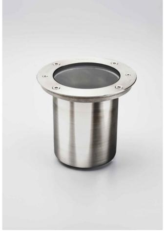
High corrosion resistance The die-cast body is made from a low copper content aluminium "primary alloy" which increases its corrosion resistance. 8µm anodisation, 15/40µm cataphoresis treatment and 100µm black polyester paint on the top, ensure protection to all exposed surfaces. Given this treatment Keplero can be installed up to 5 metres from the sea (no immersion), while maintaining a 5-year warranty 1400h resistance to salt spray testing.
