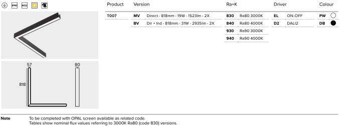
Flux values of direct+indirect versions refer to the total emission of the fixture. Related codes and accessory codes on page 237.
