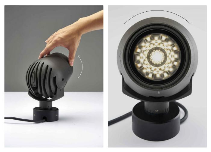
Emission can vary from Spot (20°) to Medium Wide Flood (41°) continuously with mechanical locking of the zoom on the chosen distribution. A practical graduated scale facilitates replication across multiple fixtures.
