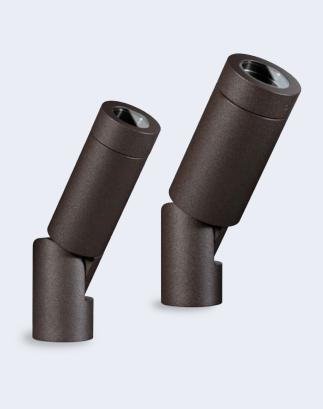
Jupiter Mini This is the simplest and most compact version in the range. It has a lens optical system for precise and defined beams. It is supplied with a stainless steel bracket that allows it to be adjusted to (+/-90°) on the vertical plane and (0-330°) on the horizontal plane. , plane.
