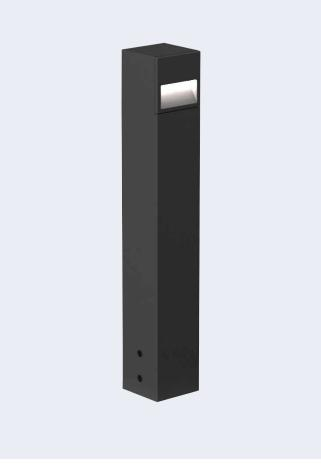
Zedge Bollard is part of the Zedge range for lighting pedestrian areas developed in collaboration with the architecture and design firm Gensler. The 24V bollard version is sleek and compact, it has a floor washer optic and is suitable for lighting small pedestrian walkways and passageways. To be completed with a special fixing system and a remote driver. Dimmable
