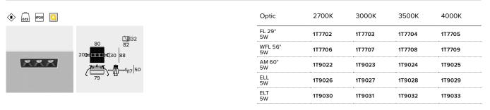
Note To be completed with an electronic or DALI driver. Values relating to the power of the fixture do not take into account the absorption of the accessory driver. This value depends on the choice of driver. Related codes and accessory codes on page 69.
